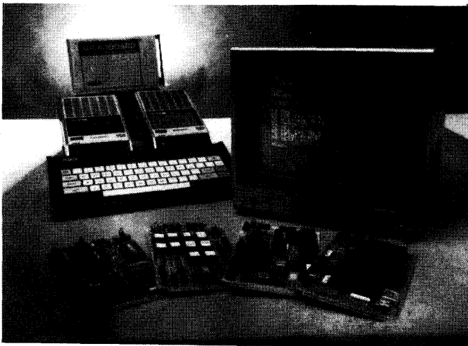
Hardware Components (5-Card Chassis shown) of Color-Enhanced Microboard Computer Development System CDP18S695V1 (For domestic use).
